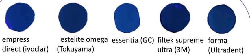
A digital photo editing program was used to analyze and record the highest B Value of each specimen.
